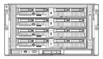
**Figure B-4.** HP BladeSystem c3000 Enclosure – Half-height server blade device bay numbering. Half-height servers should be populated from the bottom of the enclosure, in the following order: Device bays 1, 5, 2, 6, 3, 7, 4, 8.
